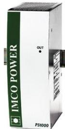
Backup power supply of PS10000.H type with 1 (2) output voltage is designed for reverse supply 12V, 24V, 48V or 24/48V up to 870W total. In case of mains failure, the connected battery provides the backup supply of connected load. The charging voltage is thermally controlled. PS1000.H 24482503 contains an additional DC/DC converter to 48V (3A) with galvanically isolation from 24V.
