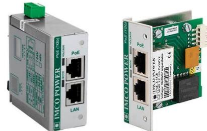
Passive PoE unit is a product, that can distribute power to devices with power supply up to 56VDC and up to 1.4A (0.35A / pair) with transmission speeds up to 1Gbps. The total power is 83W. PoE input is locked by a 1.4A fuse. The module includes a power input filter, surge protection on both the LAN and the PoE side.
