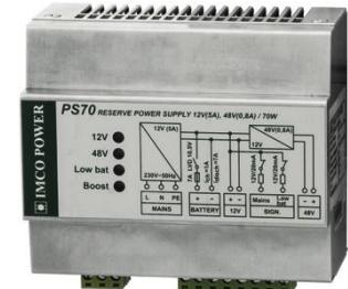
The PS70.H backup power supply is designed for reverse supply 12V/5A and 24V/1.5A or 48V/0.8A. The total output power is 70W. In case of mains failure, the connected 12V battery provides the uninterrupted backup supply on both outputs. When the battery capacity drops to a critical level, the power supply will ensure its correct disconnection. After the mains powers up, the battery will be automatically recharged to its full capacity.
