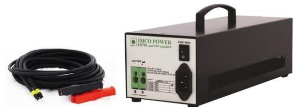
Battery charger type PS700.H is determined to charge lead acid batteries with 12V or 24V. It disposes with a converter built in the most advanced energy conversion technology with respect to maximum efficiency. The total output power is 350W (700W). Charging cables are potential free until the battery will be connected with a right polarity. When the battery is charged, charging will stop.
