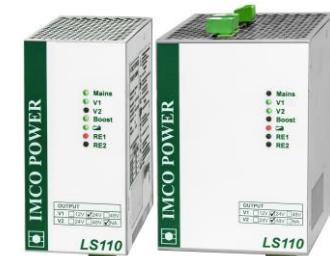
Backup power supply of LS110.H type with 1 (2) output voltage is designed for reverse supply 12V, 24V, 48V or 24/48V up to 280W total. It disposes with a converter built in most advanced technology of the energy conversion with respect to maximum efficiency. In case of mains failure, the connected 24V battery provides the backup supply of connected load. The charging voltage is thermally controlled.
