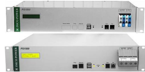
The PS1500 2U is designed for reverse supply of 24V (48V) devices with output power up to 5220W. The input voltage range is 1 (3)x 230V~50Hz. PS1500 2U allows parallel operation up to 2(3) units with respect to LVD output current. In case of mains failure, the connected battery provides the backup supply of connected load. After the mains powers up, the backup power supply ensures battery charging to its full capacity. The IUoU voltage charging curve is temperature controlled.
