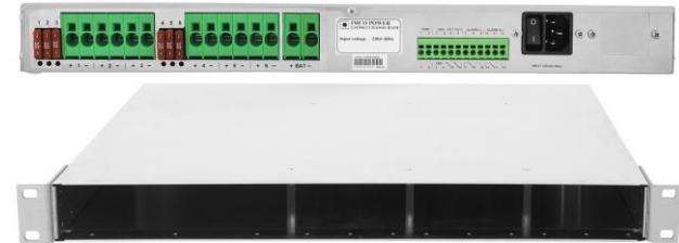
The LS1500 type power sources are designed to back up supply devices and to simultaneously charge the connected battery. In case of mains failure the connected battery continues to supply load without interruption. The power source unit is designed as a plug-in module that can be added or replaced during operation, without a need to turn the system off.
