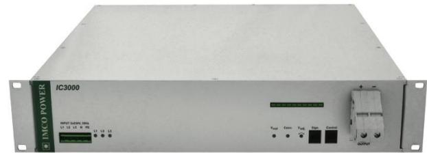
IC3000 rectifiers are used to power 24V, 48V, and 108V (110V) and 220VDC systems or as a battery charger. The input voltage of the rectifier is 3x 230V ~ 50Hz. For higher performance, units can be set in parallel. The output voltage can be set locally by a trimmer on the front panel or remotely from the PSMS4 (Power Supply Management System). IC3000 can also be used as a stand-alone power source without a connected battery.
