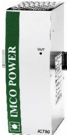
The power supply type IC750.H 22003 is intended for to supply devices with 220VDC input voltage and up to 660W. The IC750 allows long life operation in industrial environments from -25°C up to +50°C ambient temperature. Class D surge protection, short-circuit protection and galvanically isolated output are some of main features of the power supply IC750.H 22003 types additionally have an output with IU voltage characteristic.
