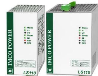
Backup power supply of LS110.H type with 1 (2) output voltage is designed for reverse supply 12V, 24V, 48V or 24/48V up to 150W total. It disposes with a converter built in most advanced technology of the energy conversion with respect to maximum efficiency. In case of mains failure, the connected 24V battery provides the backup supply of connected load. The charging voltage is thermally controlled.
